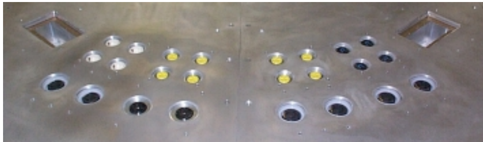
International Power Matrix Option with Flush-Mounted Receptacles and LISNs
